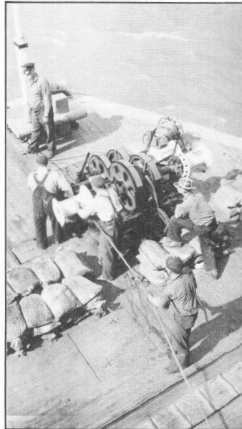
Figure 2: Unusual activities, such as "lining up" through rapids as shown in this photograph, were often the focus of photographers. As these took place on sections of the vessel not normally of interest, such photographs provide structural details of the vessel, such as the planking pattern of the foredeck, unavailable otherwise. Courtesy: Bill Lesyk.
