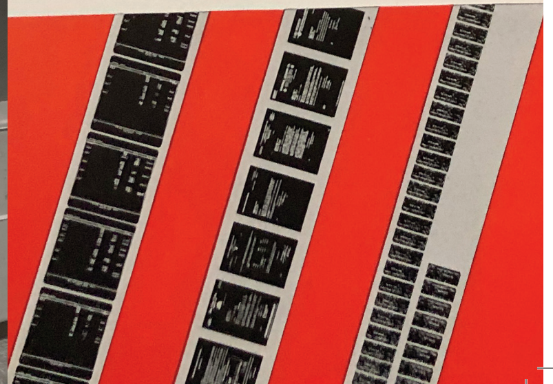
Triplex Microfilmer. General ledger sheets are microfilmed at 24 to 1 (left); or letters at 24 to 1 (center) by the Standard method; and tab cards fronts only, or fronts and backs by the Duo method (right) at 24 to 1 or 28 to 1.
